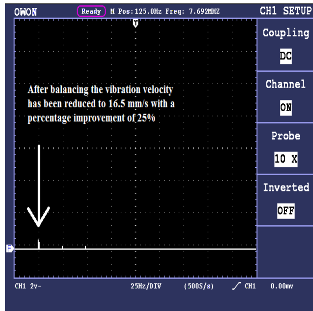
(5b). After balancing using two test runs method
