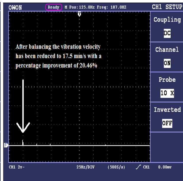
(5d). After balancing using four test runs method
